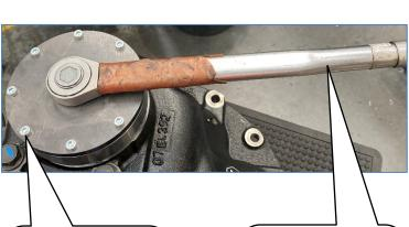
Fit the **tool plate** with 8off M6x25mm socket head cap screws (Class 12.9) at 15-17Nm to the **pump base**.
