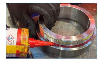
Add thread sealant (Loctite 577) and surface sealant (Loctite 518) to the Pump Base.
