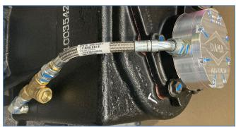
The main difference between the D170 and the D190 Full Time Pump installation, is that the D170 needs a "Pump Base" to fit the pump to the housing, the D190 does not.
