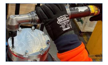
Tighten the bolts evenly in a stare pattern to <u>15 – 17Nm</u>.
